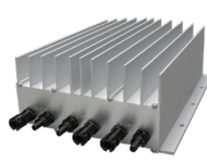
i20 String Optimizer System voltages: 750 – 1500 V Output currents: 16 – 20 A Output powers: 9.3 – 28 kW
